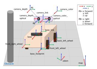
Figure 2: Frames in a Simple Robot
