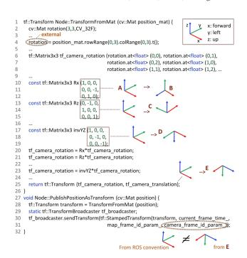
Figure 3: Example of incorrect transform between frames source: https://git.io/JtSHb, fixed source: https://git.io/JtSRt
